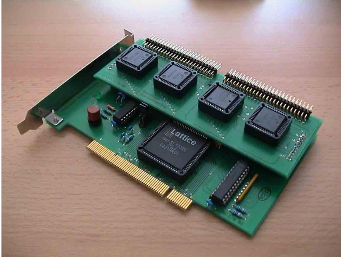
Depending of the type of track occupation feedback, you require the optical interface or the adapter interface. The optical interface provides isolated connection between model railway and computer. Hence a short circuit can not damage your computer. With this card you can connect switches (in any form). The adapter interface splits out 50 wires to connect easily to the current detection card. In combination with this card you have also an isolated connection between model railway and computer.
